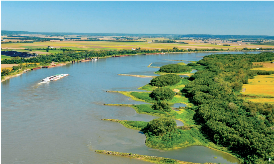
图1 美国密西西比河岸丁坝 (引自 https://news.stlpublicradio.org/ ) Fig. 1 Spur dam on the banks of the Mississippi River, USA
